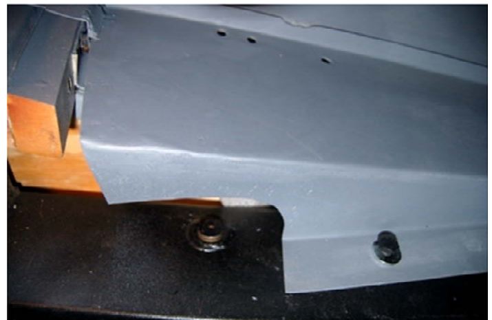
Fig.8 Fender Cutout to allow access to grease fitting on RHD MG TD and TF
