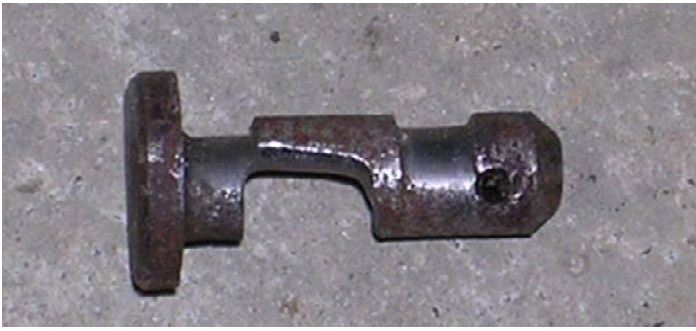
Fig. 4 Example of extreme wear on a pedal arm clevis pin.
