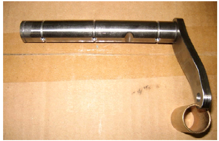
Fig. 6 Modified shaft for LHD TD/TF: showing the three lubrication grooves, the three lower lubrication holes, and the drop arm for the clutch linkage. The clearance recess for the clutch arm pinch bolt is visible between the lubrication holes for the inner frame bushing and brake arm bushing.
