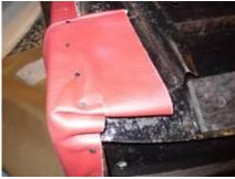
The side of the seat back is tacked under the seat bottom.
