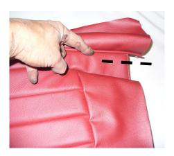
Both sides have the seam cut.. On the original upholstery the leather was cut on the dotted line but I was afraid to do this as there is then no way of going back and relieving the seam worked perfectly.
