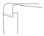
My rather crude drawing of how the horizontal side seam is cut and then overlapped on the under piece. The dotted line shows the seam that I replicated by hand. Much care is required to do this but it can be done.
