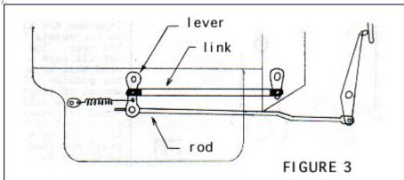
The first problem is the length of the clutch link. It should have been made adjustable but was not. As normal wear occurs, to clutch face, flywheel, throwout bearing and linkage parts, the link must travel further to the rear to release the clutch (see figure 4).
