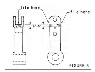
Use a round file to remove material, as shown, from both edges of the lever. This will not weaken it.
