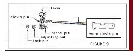
Don't worry that it's not on a flat area of the lever. Put the parts back on your car, using good new 1/4 inch clevis pins. Be sure to use the proper barrel pin, adjusting nut and locknut as shown.
