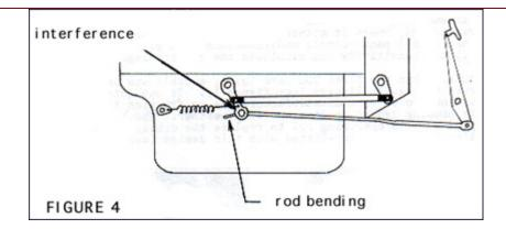
When it travels this far, the threaded end of the adjustable rod interferes with the slot in the lever. Every old lever I've seen shows signs of this interference. The result is bending and eventual breakage of the threaded rod.
