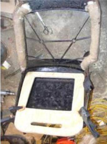
A bit of the foam must be trimmed to fit the ~~log~~ leg on the inside of the seat back.
