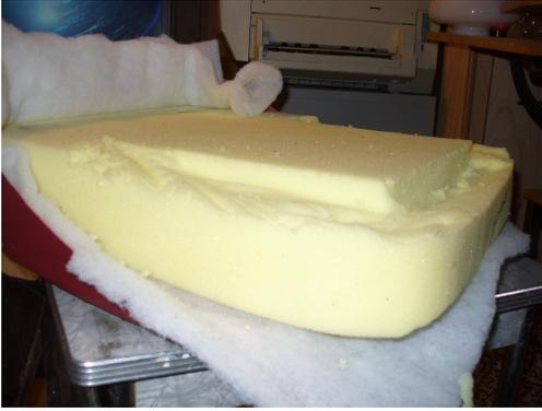
the foam must be trimmed a bit with a bread knife to fit the wooden seat bottom.
