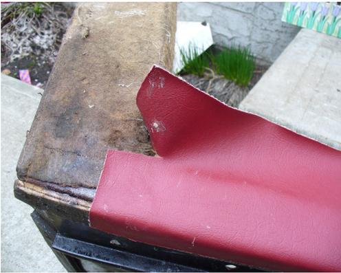
Notch the vinyl to fit around the front edge of the seat back and fold it over. Remember that the spray glue must be on both surfaces and should be allowed to almost dry before sticking. Rolling or gentle hammering with a wooden mallet will ensure a good stick were required.
