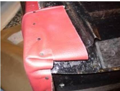
The side of the seat back is tacked under the seat bottom.
