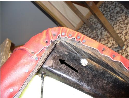
This shows the overlapped seams from the back. Each little wrinkle must be pulled further and tacked. The tighter it is the fewer wrinkles.
