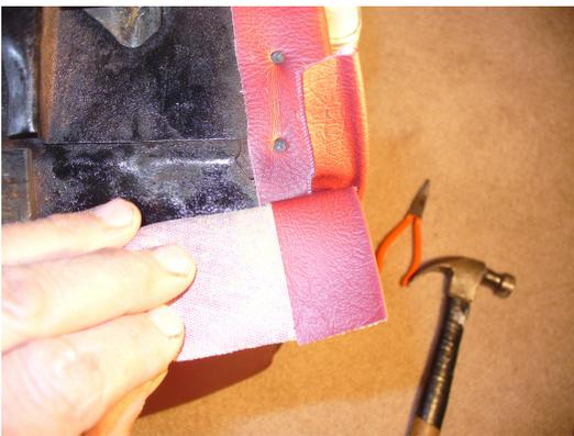
Final fit and gluing on the bottom to keep things tidy
