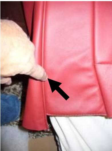
The seat back seam must be cut from the bottom up to this point to allow the center portion to pull under the seat back. At this point I then machine sewed the seam to prevent it from pulling out further but this can be done by hand.
